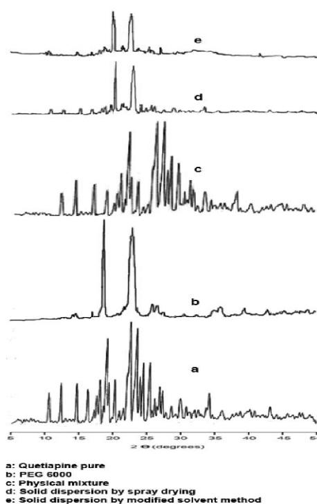
**Figure 6.** X-ray diffraction spectra for quetiapine preparations.
