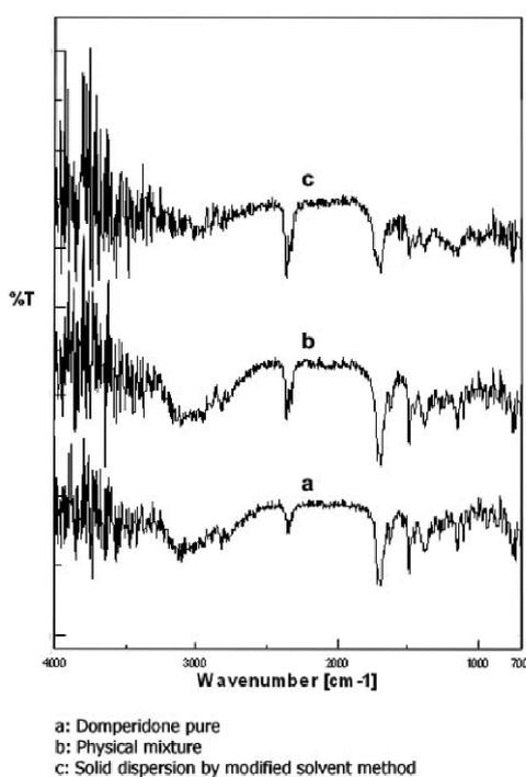
**Figure 4.** FTIR spectra of domperidone preparations.
