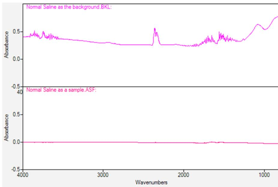
**Figure 1.** Checking the ability of the FTIR spectrometer to correctly zero the effect of background. Normal Saline is placed on ZnSe disk, dried and then the spectrum is collected as a background (top). When the spectrum of normal saline is collected as a sample, no significant infrared peak is obtained (bottom).
